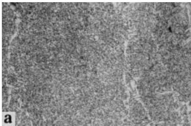
Fig. 7 Optical micrograph of (a) weld metal and (b) HAZ exhibiting acicular ferrite and bainite microstructures respectively
