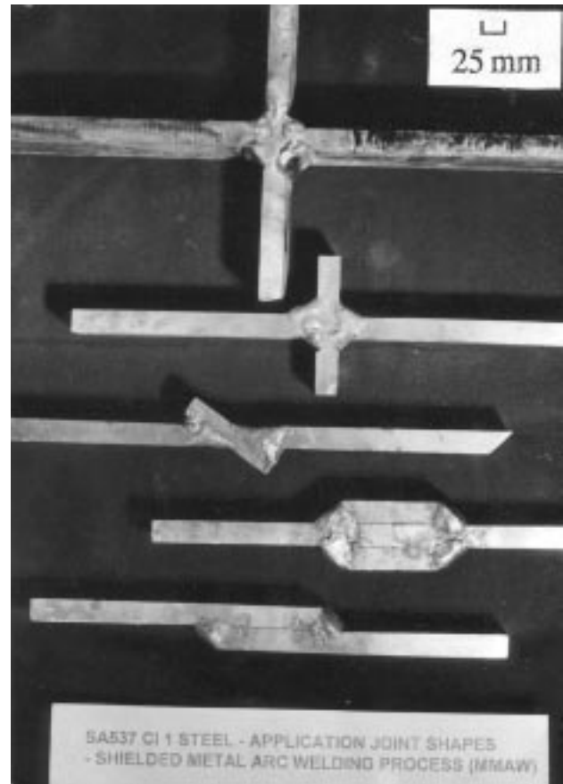
Fig. 10 Different types of weld joint configurations prepared using the SMAW process
